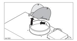
■ The non-return flap is not needed for the recirculation mode. Depending on model, it may already be fitted. Pull the non-return flap off the bracket from vent connection.
